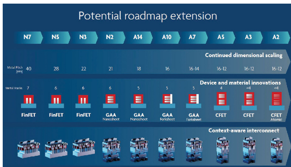
Figure 4. Imec’s new roadmap includes the continued use of 2D scaling, as well as new technologies, such as forksheet transistors and complementary FET (CFET). Source: imec, ITF World.
